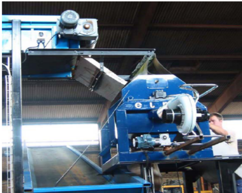
VS 800-1200 elme eddy-current separator
